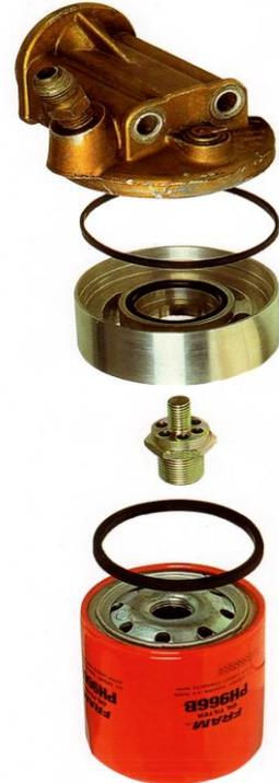
Remove the bowl containing the original filter. Remove the old filter and the sealing ring which sits in a groove in the filter head.
